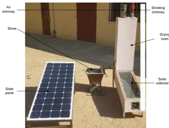
Figure 6: Photo of Biomass - Indirect Solar Dryer (BISD)
