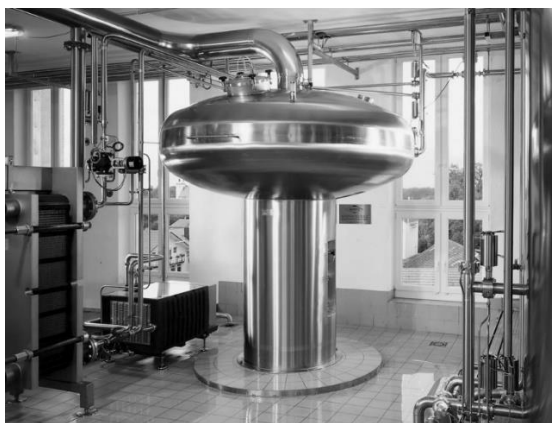
Picture 2: Schoko wort boiling system (source: Kaspar Schulz Brauereimaschinenfabrik, Bamberg, Germany)
