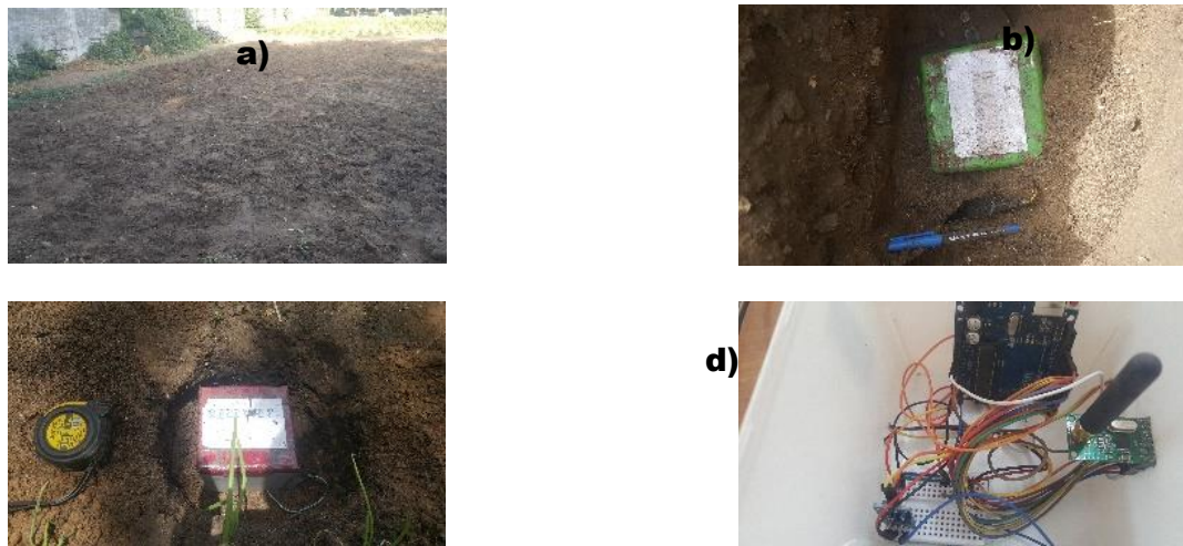
Figure 3: Overview of the experimentation field and the wireless sensor nodes. a) presents the agricultural field before the watering system is installed and the young onion plants. b) transmitter node buried under the ground in dry soil configuration. c) Receiver node buried under the ground during moist soil configuration. d) Components of the receiver node equipped with nRF905 transceiver.
